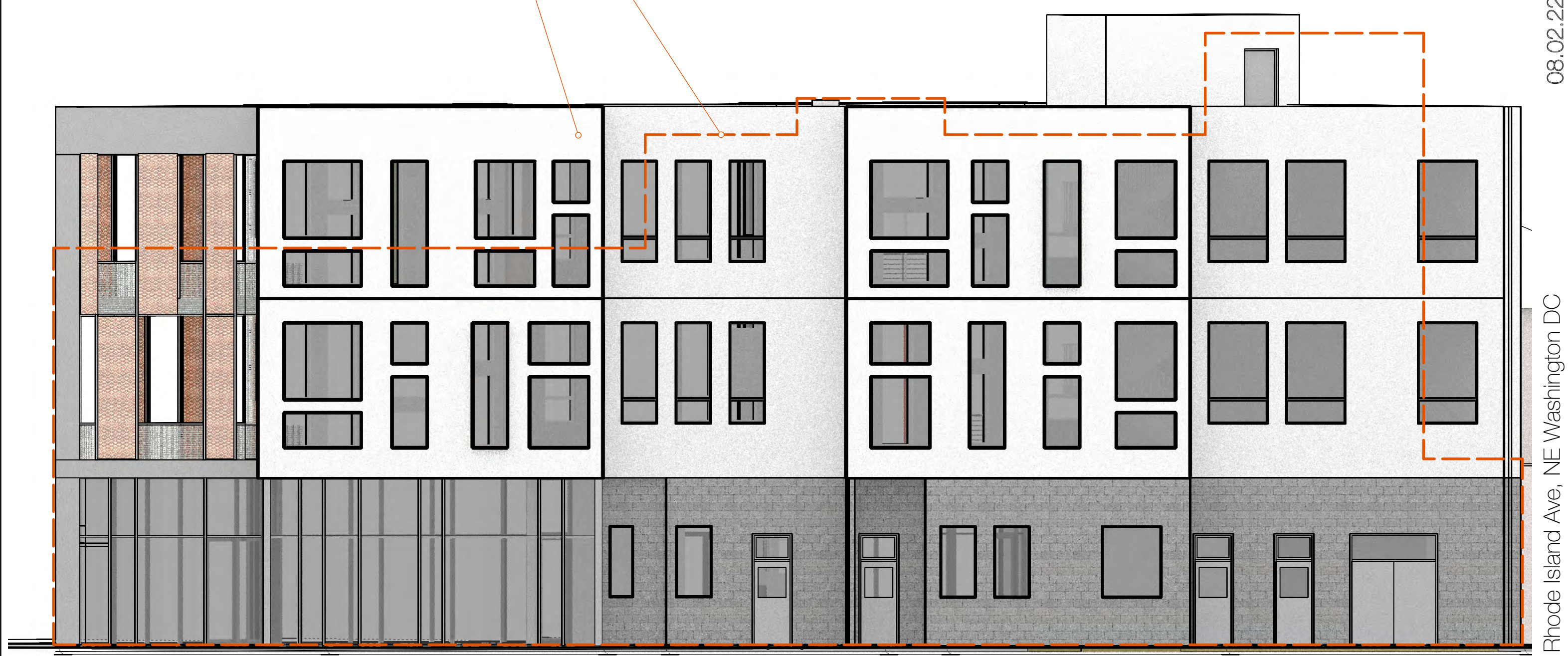
Proposed Elevation - Hamlin Street scale: 1/4" = 1'-0"
